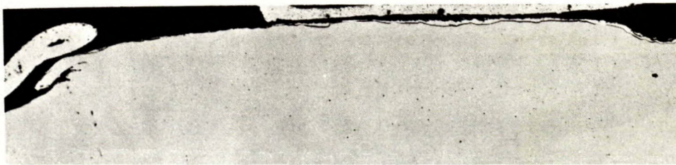
Figure 7. Microstructure of electrode KAAB showing relatively minor mushrooming at edge of contact surface. X100, Ammonia-hydrogen peroxide etch.
