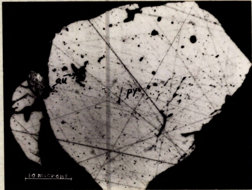
Figure 1. Two particles of native gold (au) associated with a grain of pyrite (py). The black areas are bakelite mounting medium. X500.
