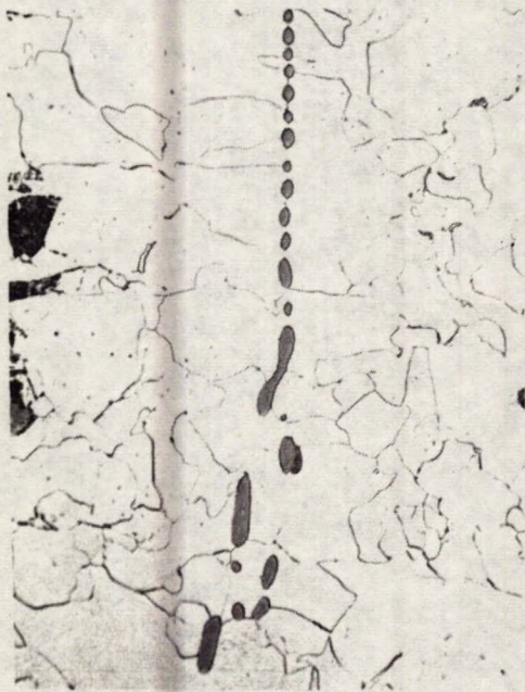
Figure 15. Sulphides forming the grain boundary film in a region remote from the tip of the crack. Corrosion and oxidation have not started in this region.
