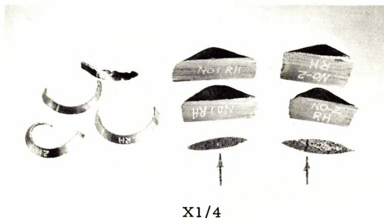
Figure 9. Samples from Blades No.1 R.H. and No.2 R.H. Metallographic examination was made on sections cut along the centre axis of the two boat samples, illustrated (arrows). One of the sections intersected the crevice visible in the boat sample at the right of the picture.
