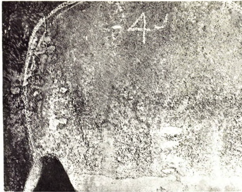
Figure 3. No. 3 R.H. Blade Surface. Forward Surface. Opposite to that shown in Figure 2. "Weld deposits" have not been attacked during service. Minor quantities of crevice defects are present on this surface.
