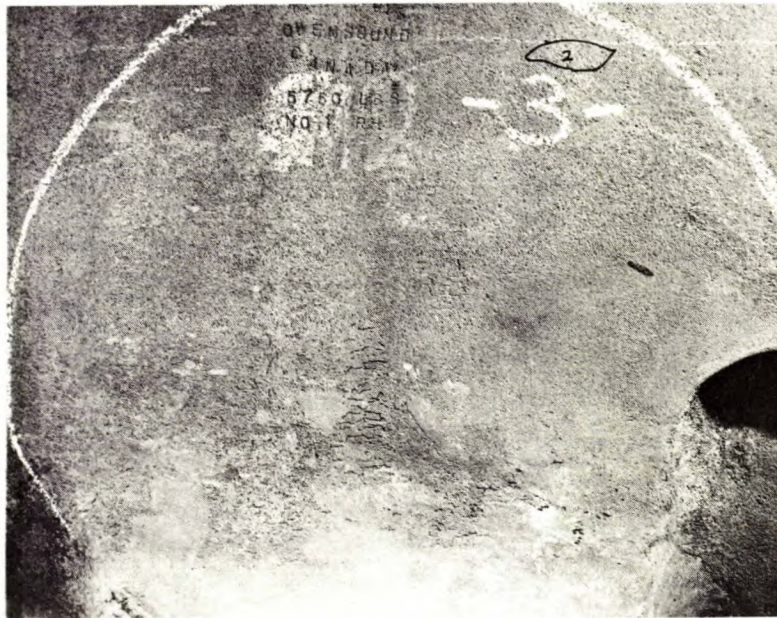
Figure 3. No. 3 R.H. Blade Surface. Forward Surface. Opposite to that shown in Figure 2. "Weld deposits" have not been attacked during service. Minor quantities of crevice defects are present on this surface.
