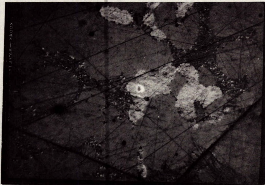
Figure 1. Polished Section of Macassa Bar Magnification: 350 X (Straight lines are polishing scratches)
