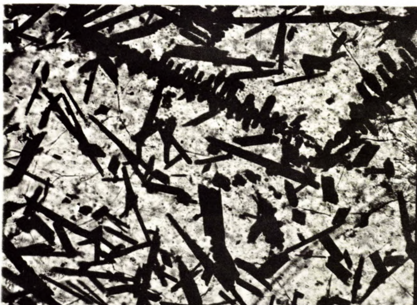
Figure 4. Photomicrograph of Thin Section of Macassa Slag Magnification: 270 X
