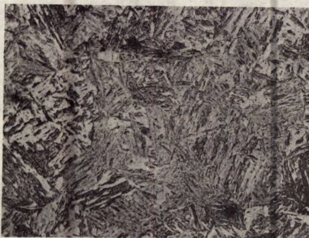
Figure 5. Shows tempered martensite structure found near outside edge.
