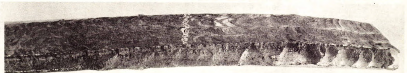
Figure 6 - Small cavities and other markings in fracture around circular patch.
