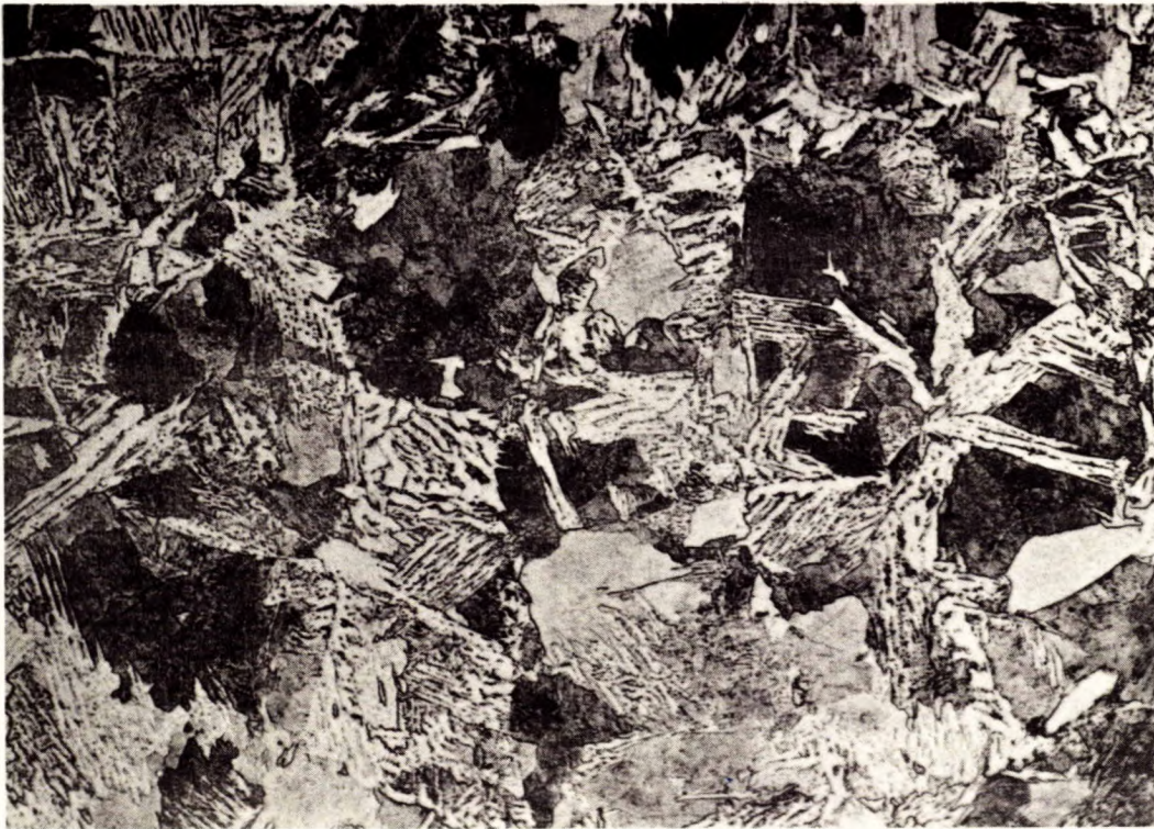
Figure 12 - Structure of typical untempered heat-affected zone adjacent to a girth weld.
