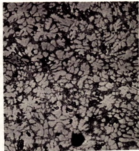
Figure 14. Structure of manganese-containing Zamak 5 (CM).
