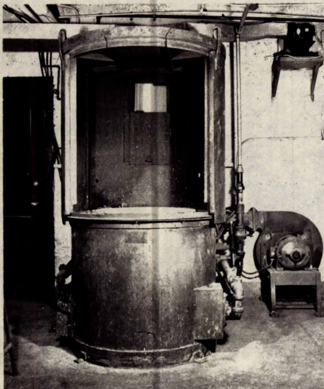
Figure 3. Fisher sulphur dome furnace (Dome removed).
