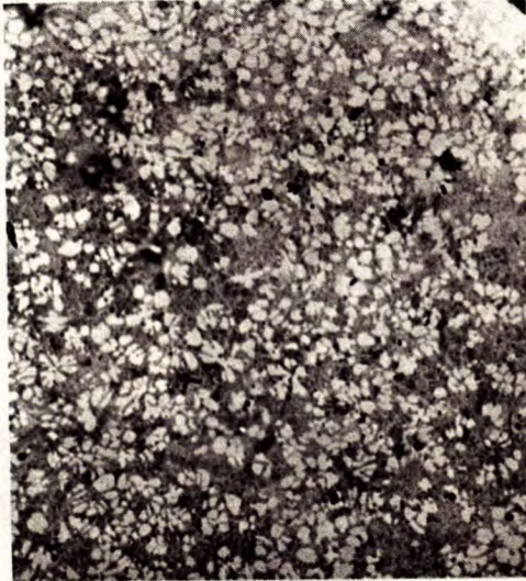
Figure 11. Structure of impact bar from cast MD. (0.06% Mn)
