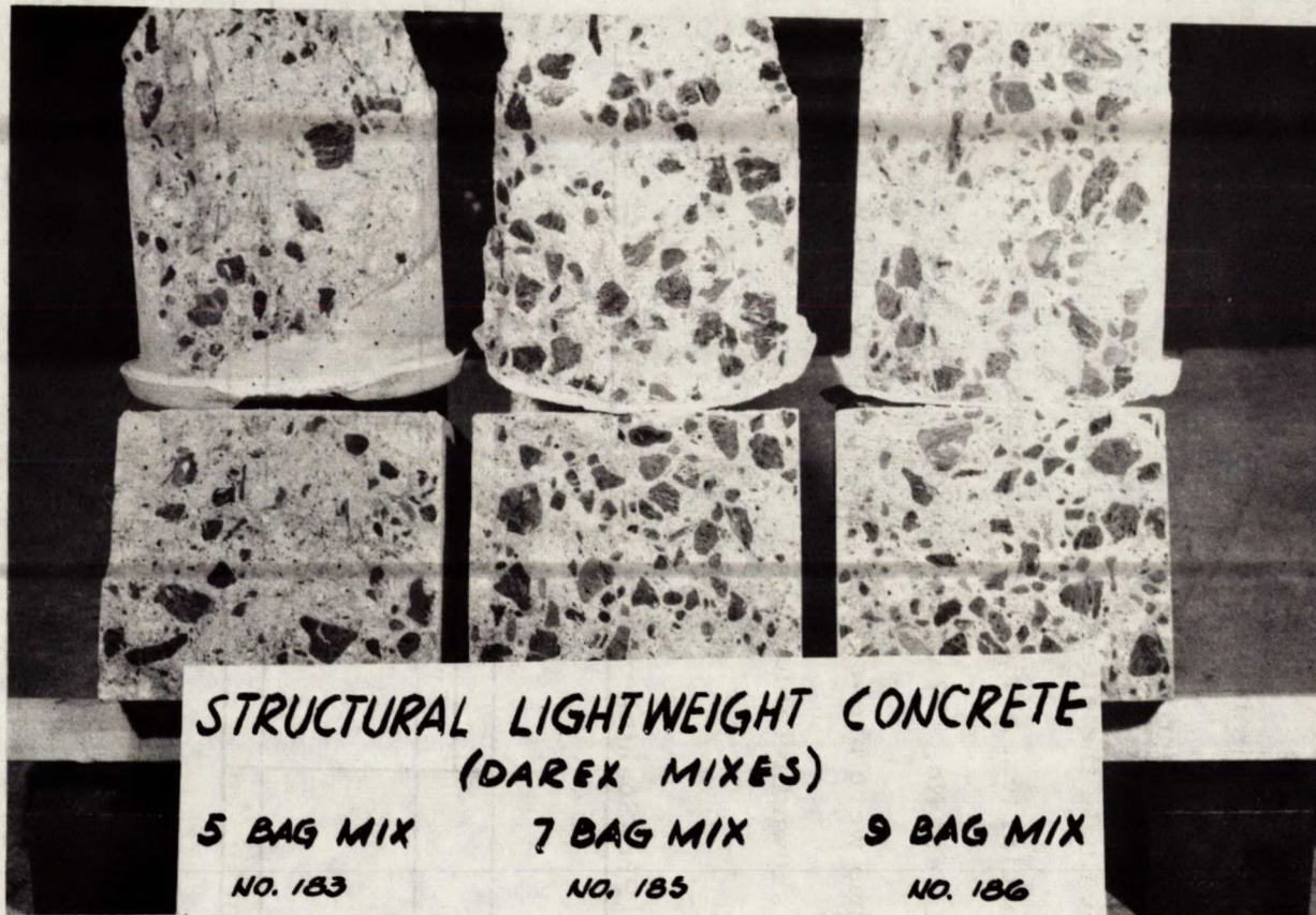
Figure 1. Broken test specimens from Series 1. Beam fractures are shown in the lower row, cylinder fractures in the upper row.
