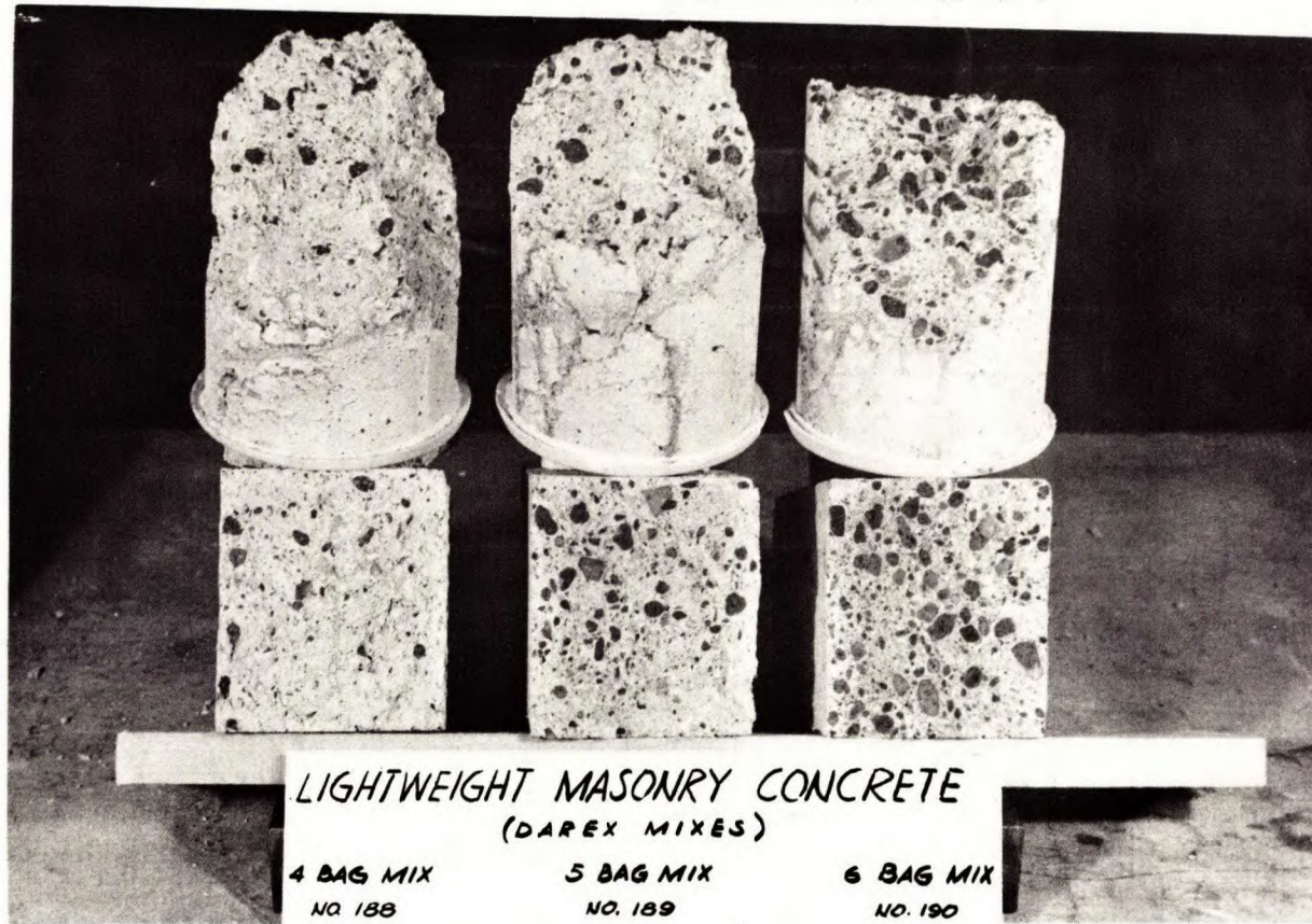
Figure 3. Broken specimens of masonry concrete. Both beams (lower row) and cylinders show a greater proportion of broken aggregate in the richer mixes.
