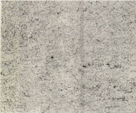
X500 (a) Etched in 2% nital
