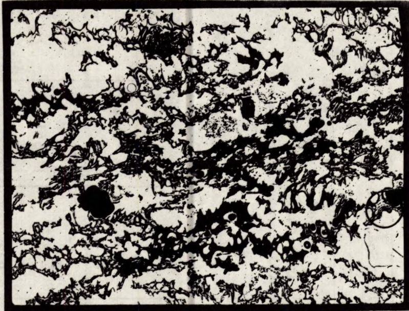
Figure 4. Photomicrograph of section of Featherrock, showing glass (shards) and porous structure. The darker glass is part of a dark band traversing the specimens; here, minute inclusions are more abundant. Magnification 6X.
