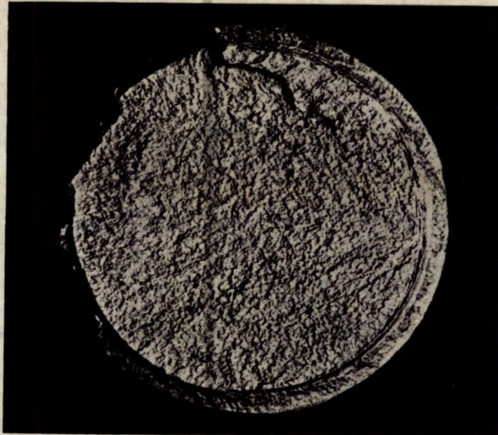
Figure 1. Surface of Fracture in a Bolt from Steel Sheet Piling.
