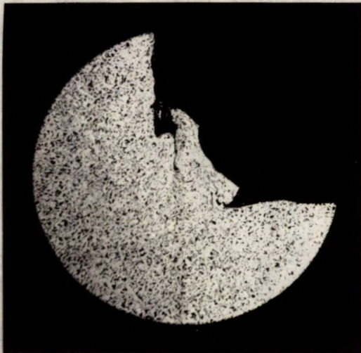
Figure 6. Section of Keyway near Fracture
