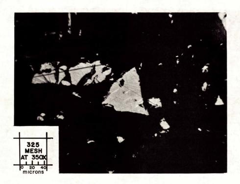
Figure 1. - Photomicrograph showing particles of pyrrhotite (grey) in bakelite (black), Cave Zone ore fine fraction; note tiny blades of pentlandite (?), white, in triangular grain of pyrrhotite near centre; straight black lines are polishing scratches.
