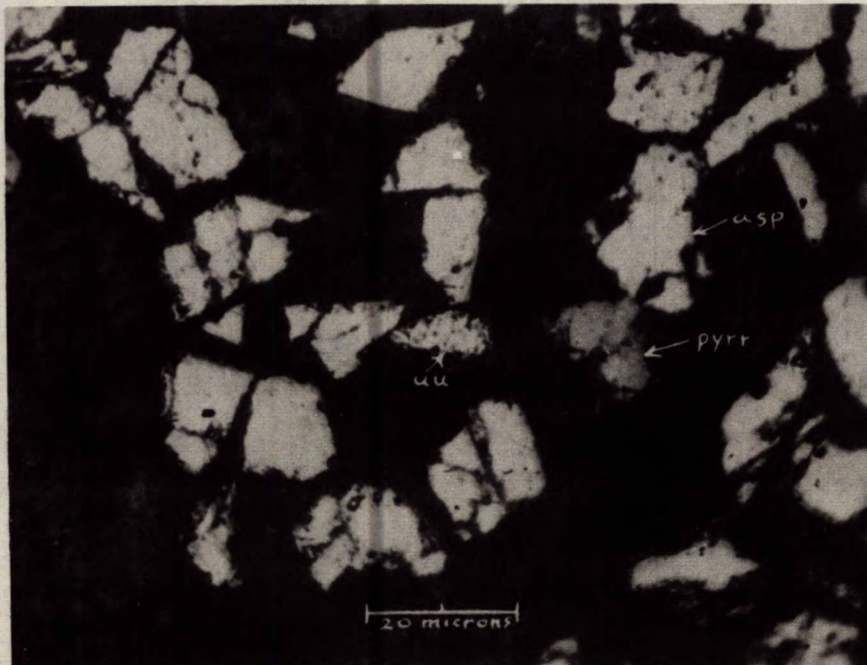
Figure 2. Native gold (au), pyrrhotite (pyrr) and arsenopyrite (asp). The unmarked grains are pyrite. Minus 28 plus 20 micron size. X1000.
