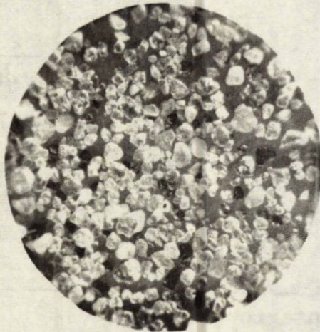
Figure 1 - Penetanguishene Sand. X20
