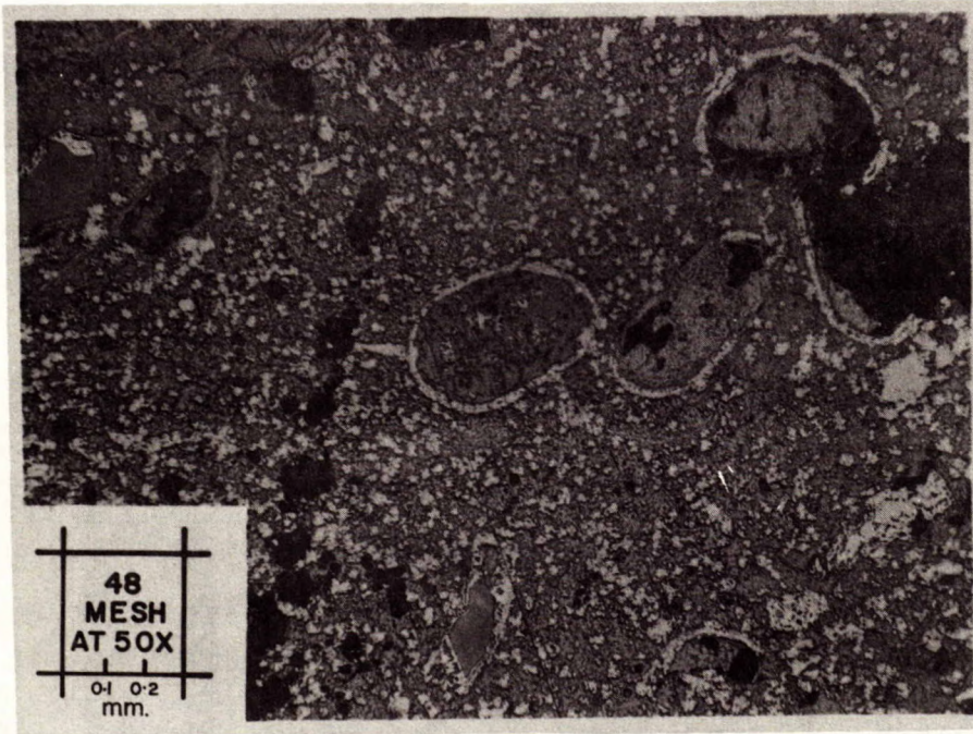
Fig. 1. - Photomicrograph of polished section of ore, showing oolites rimmed by goethite (white) in a matrix of glauconitic silicate (grey) with disseminated goethite. The oolite in the centre of the photograph consists largely of calcite; the others, largely glauconitic silicate. Pits are black.
