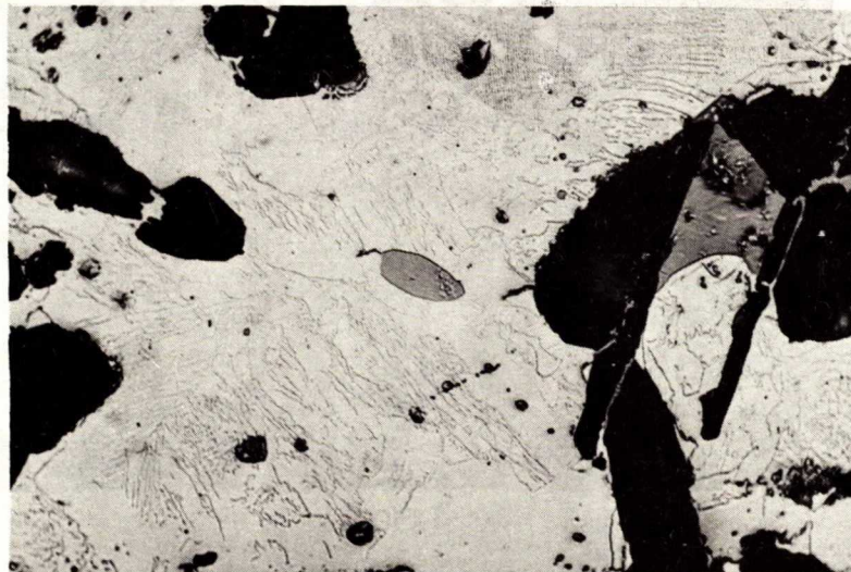
Figure 12 Sample 13-2 Etched 15 seconds in 4% Picral.
