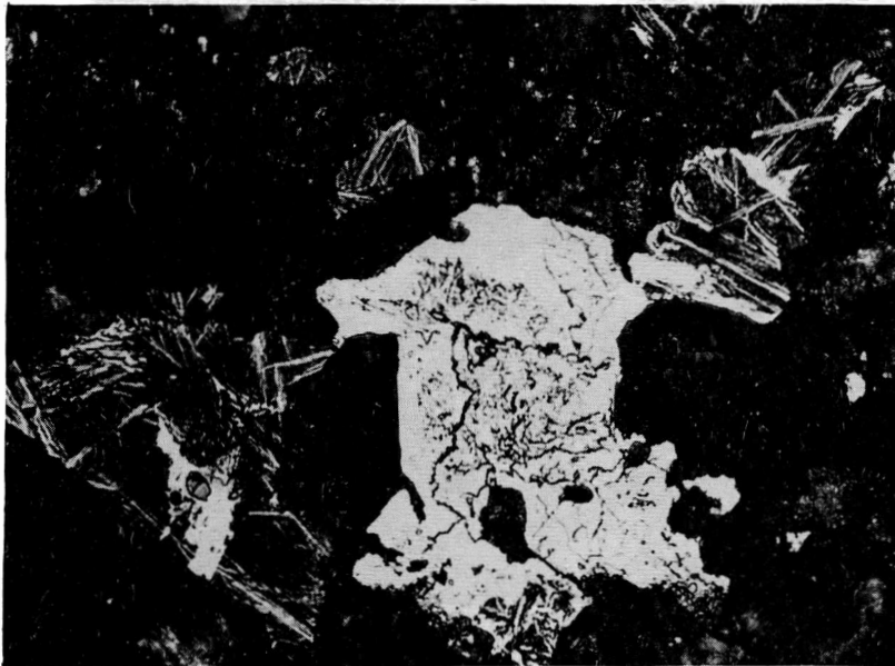
Figure 22. Sample 13-2 Etched 1\frac{1}{2} minutes in boiling alkaline sodium picrate.
