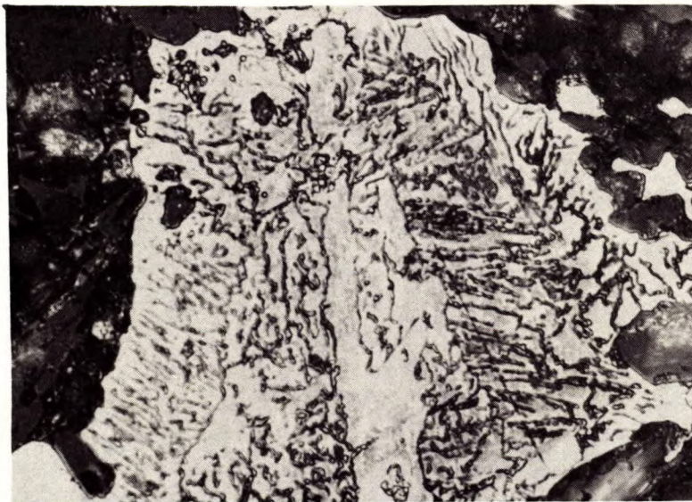
Figure 16. Sample 13-2 - Etched 1\frac{1}{2} minutes in boiling alkaline sodium picrate.
