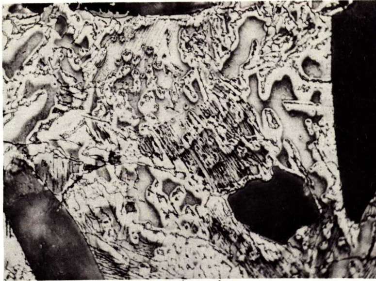
Figure 27. Ferrite-Pearlite Area Inside Crust Sample 1-1. Etched 40 seconds 4% picral.
