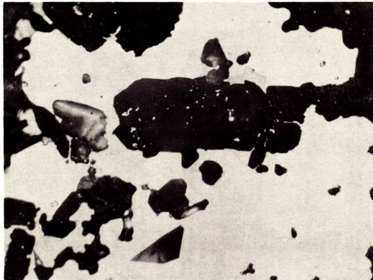
Figure 7 - 13-2 As-Polished Enstatite, sulphide mineral and alpha iron.
