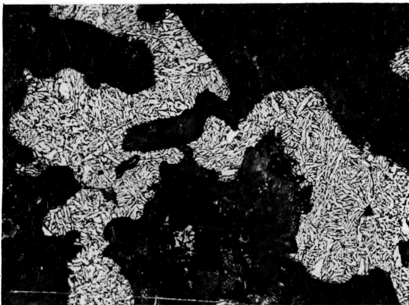
Figure 37. Sample C \frac{1}{2} minute in boiling alkaline sodium picrate.
