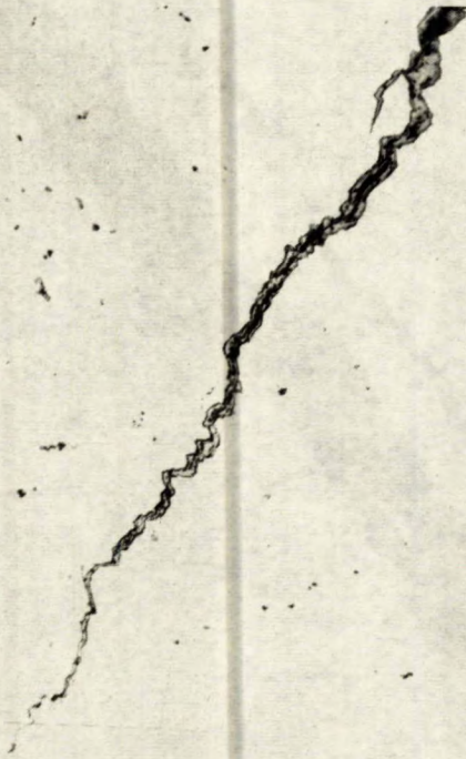
(Unetched; magnification X100) Figure 7. - Photomicrograph of the bottom position of the major crack shown in Figure 6A.
