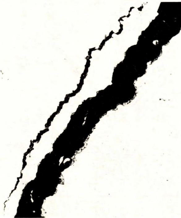
(Unetched; magnification X100) Figure 6A. - Photomicrograph showing crack area. Fine particles are sulphide.
