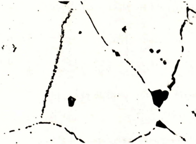
- (Mag. X500 - Etched in 10% Oxalic acid, 5 amps, 5 sec) Figure 7 - Alloy #40, held 10 hours, 1950°F, air cooled, annealed at 1390°F, 500 hours.
