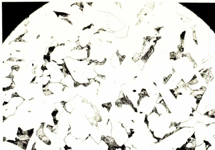
Figure 4. - Axle C - taken at right angles to fracture face. (X100; Etched in 2% Nital)
