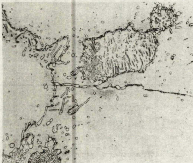
Figure 2 - Shows carbide at grain boundaries as well as the needle-shaped carbide typical of as-cast manganese steel.
