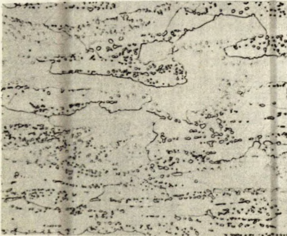
Figure 6. - A-1022-C-111211-19(4) Same as Figure 4 but at higher magnification. Illustrates incomplete spheroidization in finished-wire sample.
