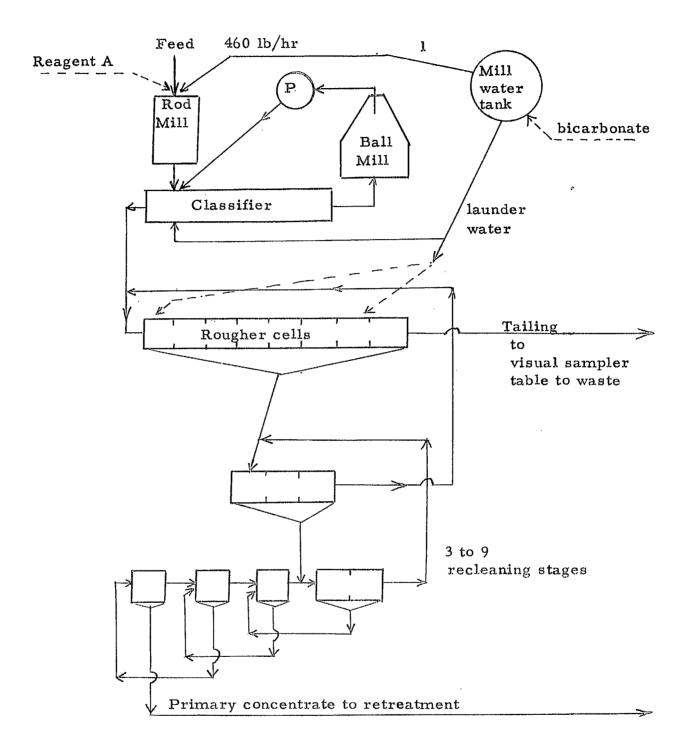
Figure 1 - Flowsheet for Continuous Flotation of Oka Ore.
