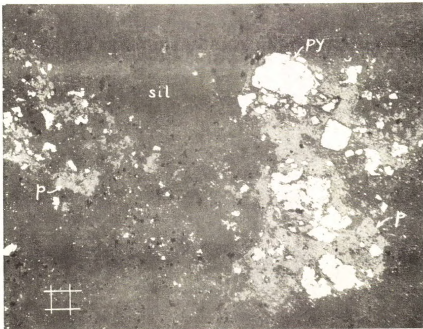
Figure 5 - Irregular masses of pitchblende (p) with inclusions of pyrite (py) in siliceous gangue (sil). Sample 1101.
