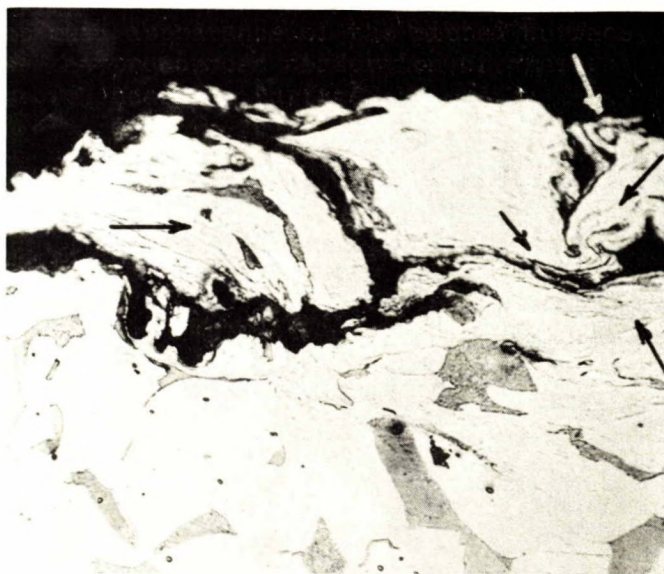
Figure 7. - Photomicrograph showing the cross-sectional appearance of the pitted surface. Note the pronounced distortion of grains (arrows) near the surface.
