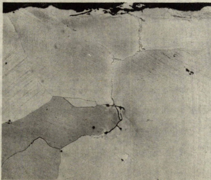
Figure 1. - Area at surface showing large grain size and patches of carbide concentrated mainly at the grain boundaries.
