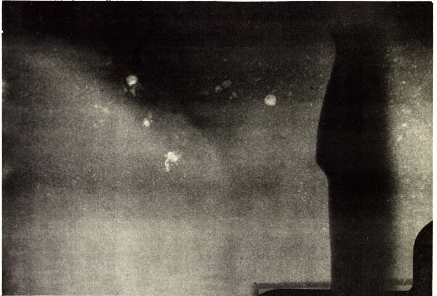
Fig. 8. - Print from a radiograph of the smallest (approximately 20 in. x 17 in. x 7 in. deep) cover showing unsound region.
