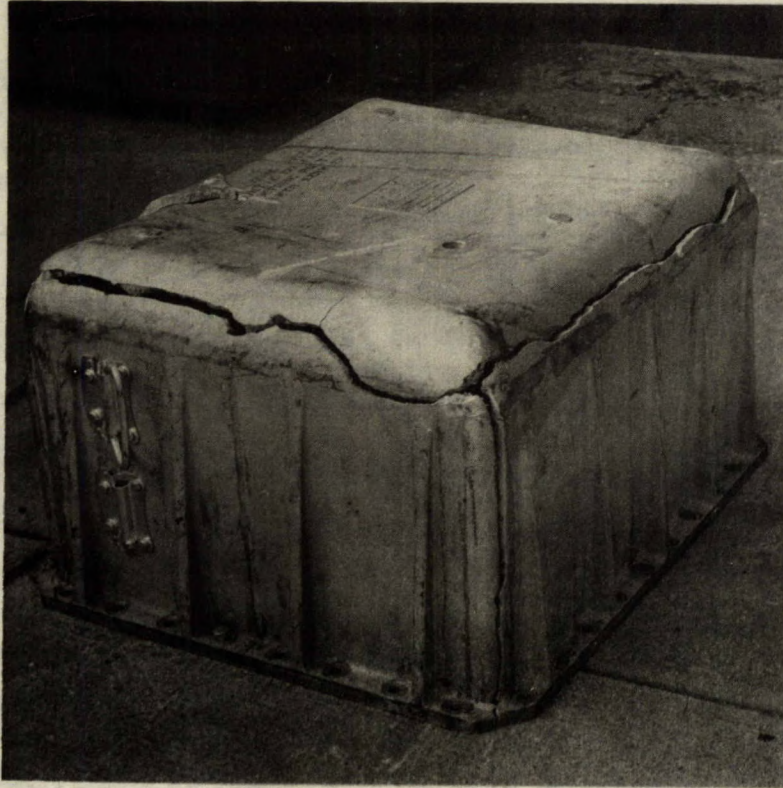
Fig. 1. - View of the parts of the broken circuit-breaker cover reassembled roughly in their original relative positions. Note that failure has occurred at the junction of each face. There are several smaller cracks in the upper face.
