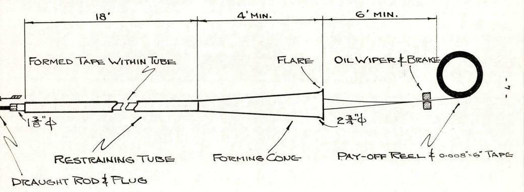
FIG 2. DIAGRAMATIC SKETCH OF FORMING GEAR
