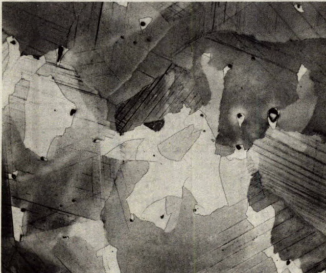
Figure 1. - Microstructure of sample #1 showing relatively small grain size.
