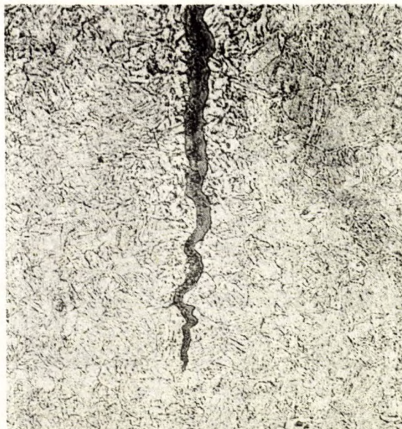
Figure 5. - Tip of the transverse crack. The presence of decarburization and high temperature oxide close to the tip of the crack indicates that in service the crack did not propagate.
