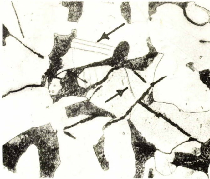
Figure 15. - Intercrystalline cracks and twinning of ferrite grains. Twinning of ferrite grains is marked by the arrows.
