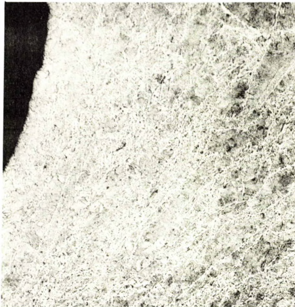
Figure 12. - Rivet "D" - fillet between point and shank. The driving temperature and the cooling rate after driving were successful in avoiding cold work, grain growth, or a severely quenched microstructure.
