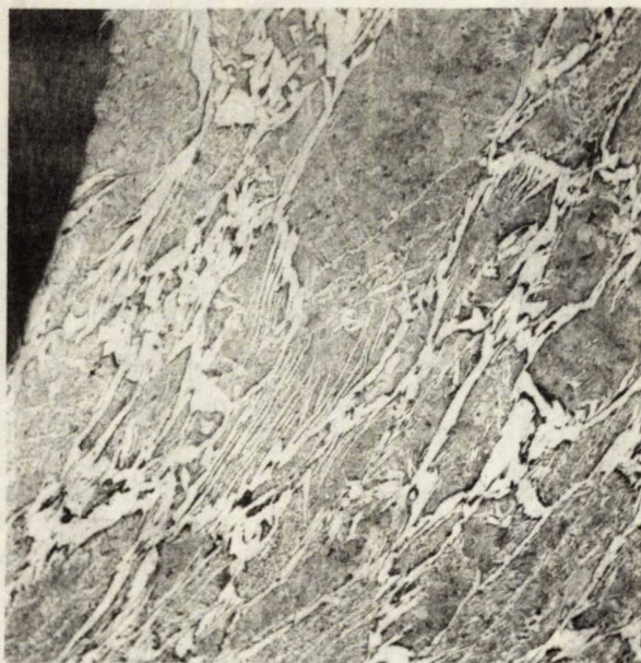
Figure 13. - Rivet "E" - fillet between point and shank. The structure is similar to that of Figure 12, except that this rivet was probably driven hotter than rivet D, resulting in a slightly coarser grain size.
