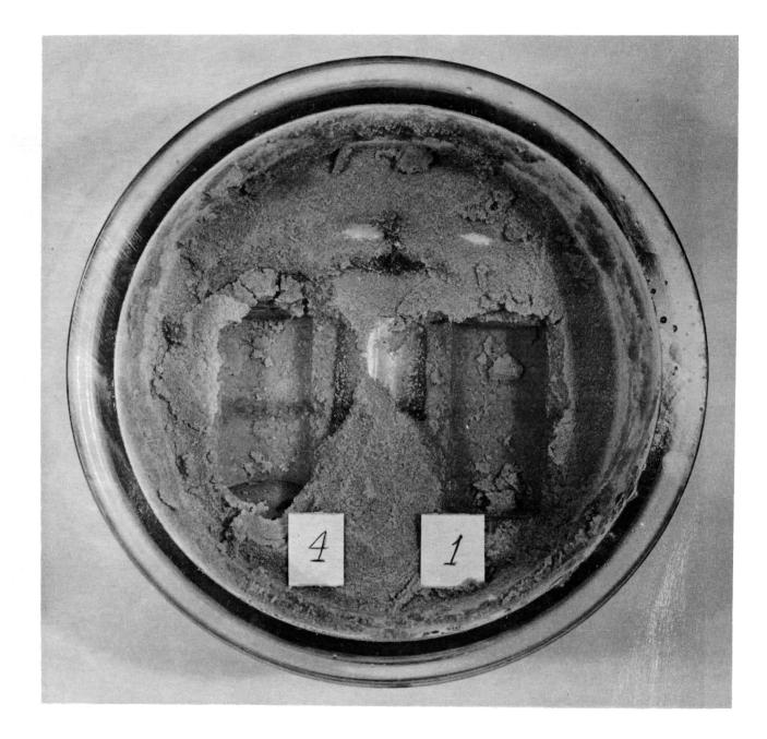
Figure 2 - Depressions left in moist sand by specimens Nos. 1A and 4M. Tops of specimens 2A and 3M also visible.
