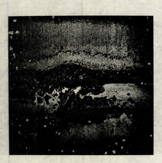
Figure 4 - Another region of same interior weld shown in Figure 3. Solidified flux and corrosion product not removed (6X).
