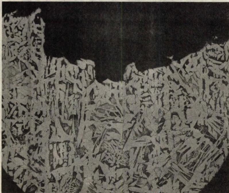
Fig. 12. - Microstructure across fractured surface of Sample EH 3. (X100. Etched in 2% nital.)
