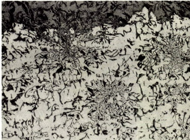
Fig. 2. - Photomicrograph of surface of Sample A, showing some penetration along the graphite flakes.
