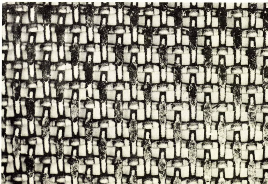
Fig. 6. - Body of the wire cloth sample remote from the mend.
