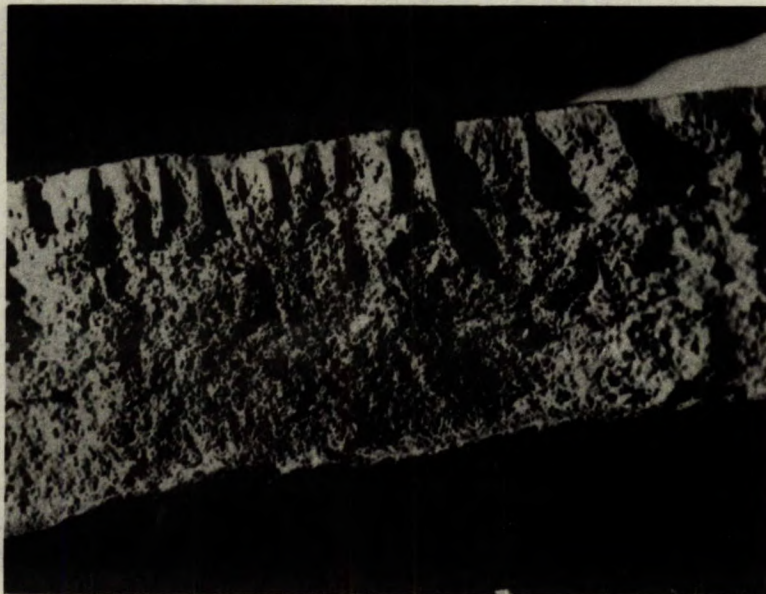
Fig. 5. - Same as Fig. 4, but the fracture surface is more coarsely crystalline.
