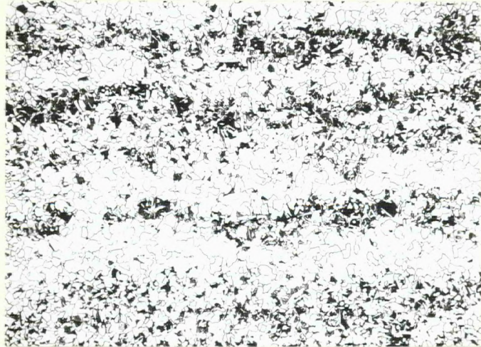
Longitudinal Section, Specimen B, Heat 10519. (X40; etched in 2% nital)
