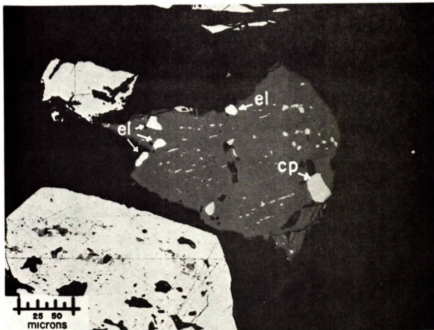
Fig. 2. Photomicrograph of the sink product from the 35 to 48-mesh fraction of the head sample. The field shows four small grains of electrum (el) in a grain of sphalerite (dark grey). The sphalerite also contains numerous small blebs of chalcopyrite (cp). The large white grains are pyrite.
