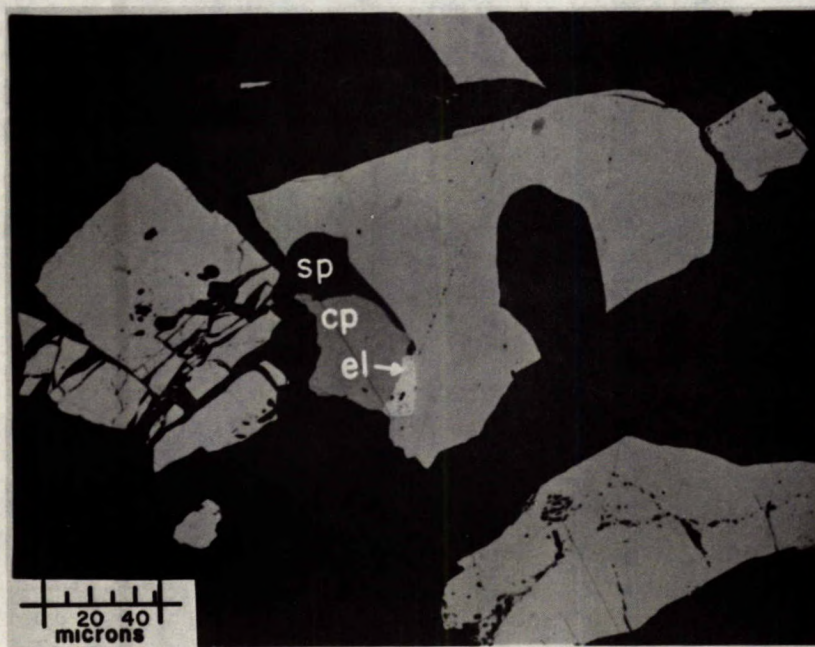
Fig. 4. Photomicrograph of a polished section of the sink product of the 65 to 100-mesh fraction of the head sample. The field shows a grain of electrum (el) occurring at the interface between pyrite (greyish white) and chalcopyrite (cp). A small inclusion of sphalerite (sp) occurs in the pyrite.
