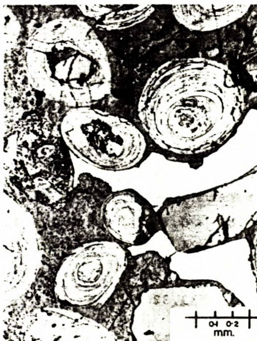
Figure 1. Photomicrograph of the Clear Hills iron ore showing oolites embedded in the "earthy" matrix. The oolites have variable quantities of goethite (white) and some have quartz cores (dark grey). The interstitial earthy matrix has siderite inclusions (light grey) and has many shrinkage fractures. A goethite veinlet (white) is seen in the middle of the photograph.
