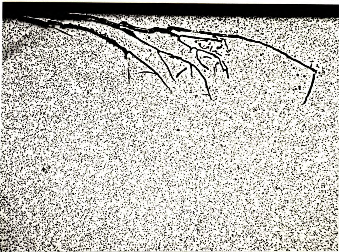
Figure 13. These flaws occurred cyclically with that shown in Figure 12(d). Section (a) above occurred 68 in. before and (b) 68 in. after the flaw in Figure 12(d).
