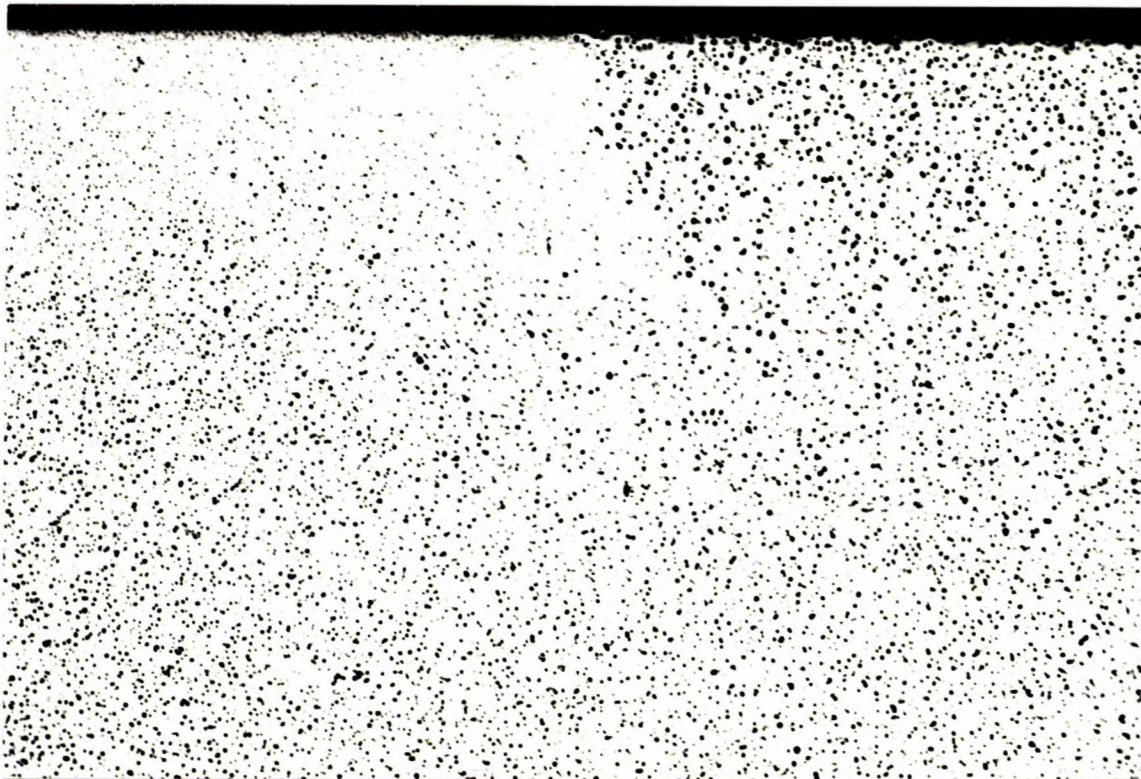
Figure 19. Two examples of abrupt changes in graphite nodule density occurring below a surface lap mark. Unetched X20
