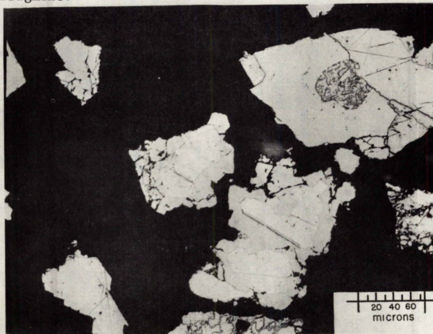
Figure 13. Photomicrograph of two native silver grains (white) enclosed in arsenides (centre of photo), native bismuth associated with an arsenide (top right), and a liberated native bismuth fragment (lower left).
