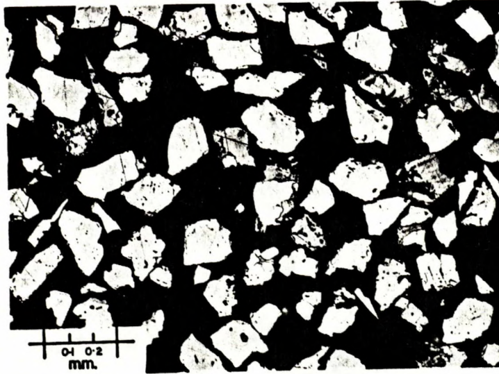
Figure 2. 65 to 100-mesh, 3.70-gravity sink fraction showing pyrite (light grey) and chalcopyrite (grey) grains. Some of the chalcopyrite is locked in pyrite.
