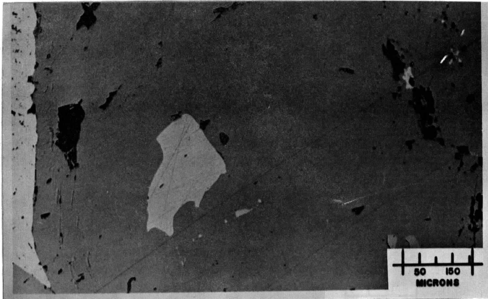
Figure 3. Photomicrograph showing galena inclusions in sphalerite. The light-coloured area on the left is pyrite. Black areas are pits.
