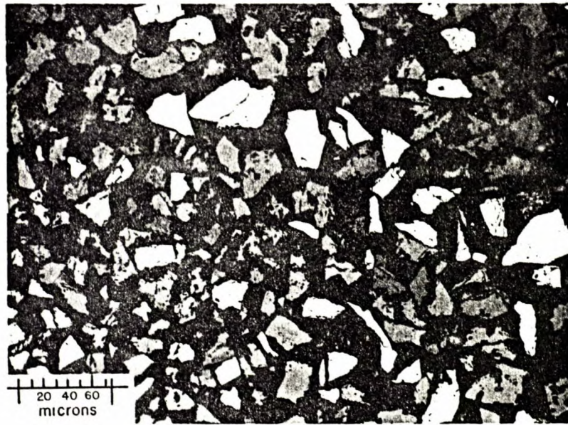
Figure 5. Photomicrograph of the sulphide grains (white) in the coarse Ta cleaner concentrate of Test 9.
