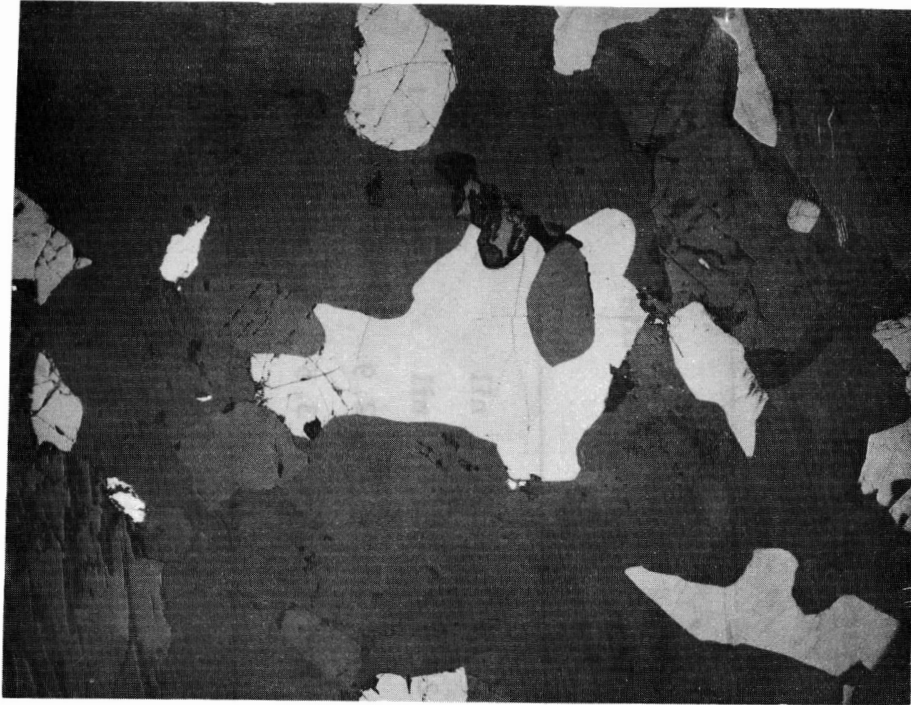
Figure 1. - Photomicrograph of the ilmenite ore showing disseminated ilmenite and magnetite (grey, not resolved in this photograph) and pyrite (white) (X 80).
