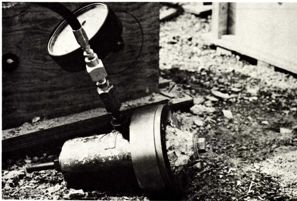
Figure 10. The 30-ton tension ram immediately after the pull-out test. The dial gauge can be seen at the top.
