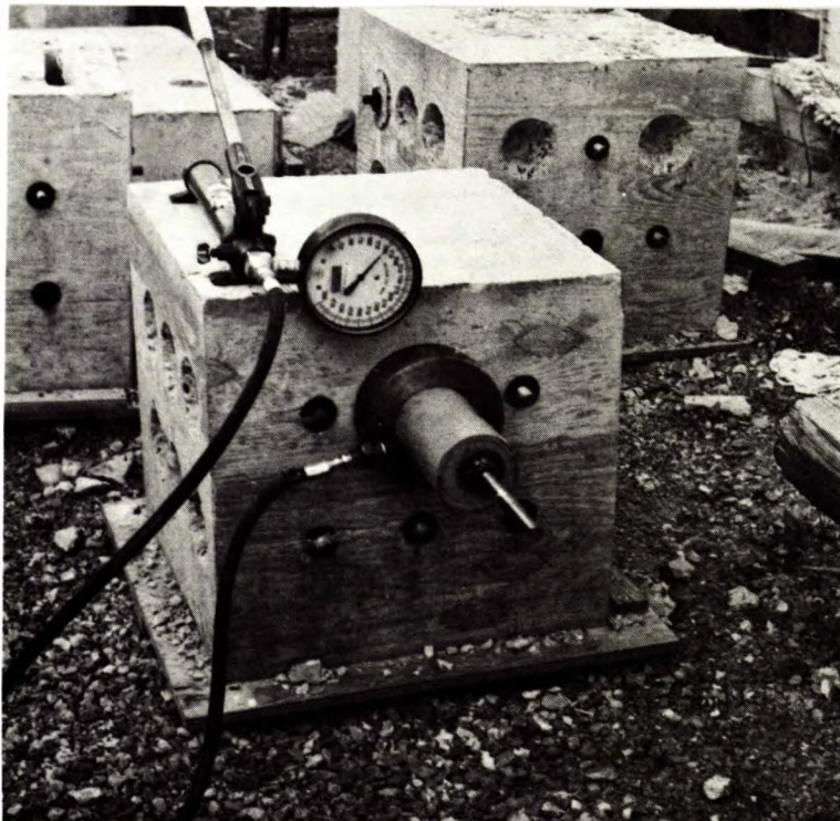
Figure 7. A view of the 30-ton tension ram being positioned on the pull-out assembly.
