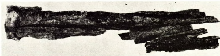
(a) As Received, Carburized, Wrought Iron Spike.
