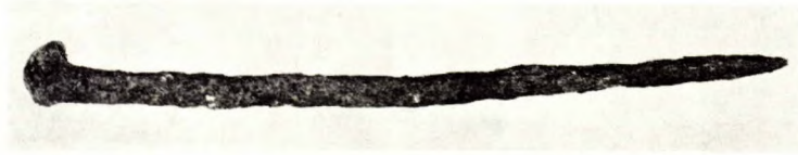
(a) As Received, Land-Recovered Spike. (Round Head Hand Made).
