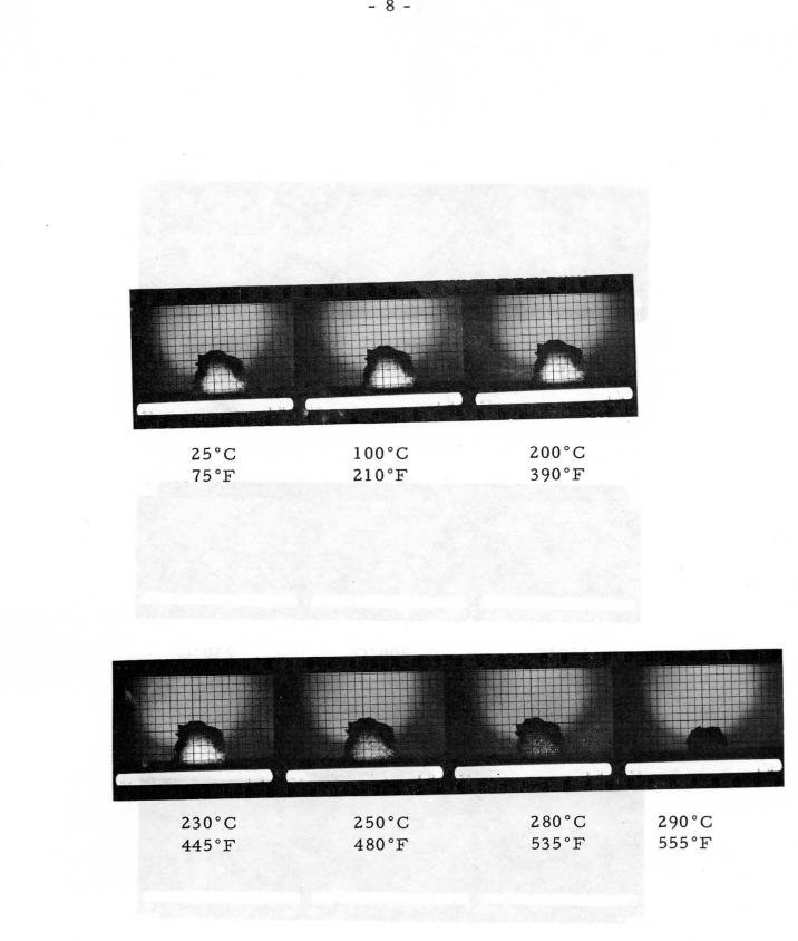
Figure 5: Nitrogen Atmosphere 40-minute heating period.
