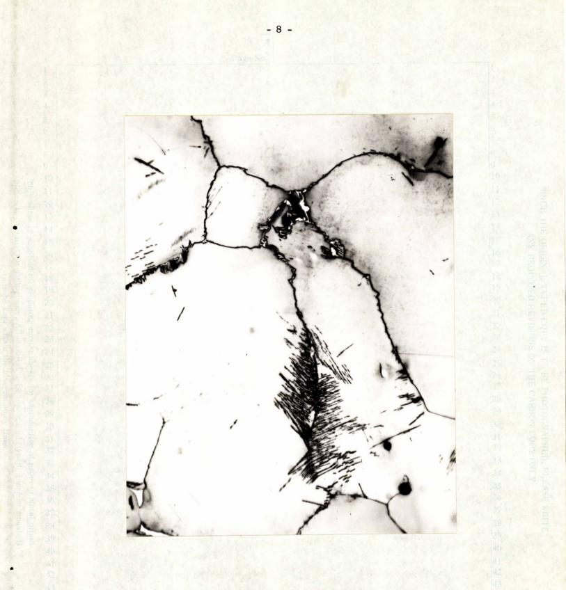
Figure 1. Non-magnetic steel, etched in 2% nital, showing large austenite grains with "massive" and acicular carbides. X600
