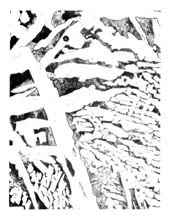
Figure 3. Magnetic sample showing white ferrite and dark pearlite. X600
