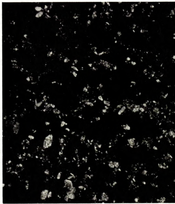
Minus 65-mesh, washed, ground to 5000 cm 2 /g, and calcined.
